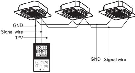
1 When installing more than 2 units of air conditioner to one wired remote controller, please connect as the right figure.
