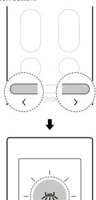
3 Press the < or > button to adjust airflow direction. Then press the Function button.
