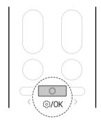
3 Press the < or > button until the below icon flashes at the bottom of the display screen. Then press the **Function** button.
