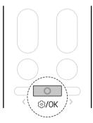
3 Press the < or > button until the below icon flashes at the bottom of the display screen. Then press the Function button.
