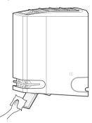
4 Press and hold the ₹ button for about 5 seconds to close the air deflector.
