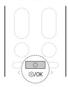
Press the < or > button until the below icon flashes at the display screen. Then press the Function button.
