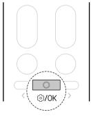
**3** Press the **<** or **>** button to set the below icon flashes at the bottom of the display screen. Then press the **Function** button.
