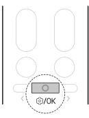
Press the < or > button until the below icon flashes at the bottom of the display screen. Then press the **Function** button.
