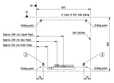
Connecting gas/liquid pipe, drain hose
